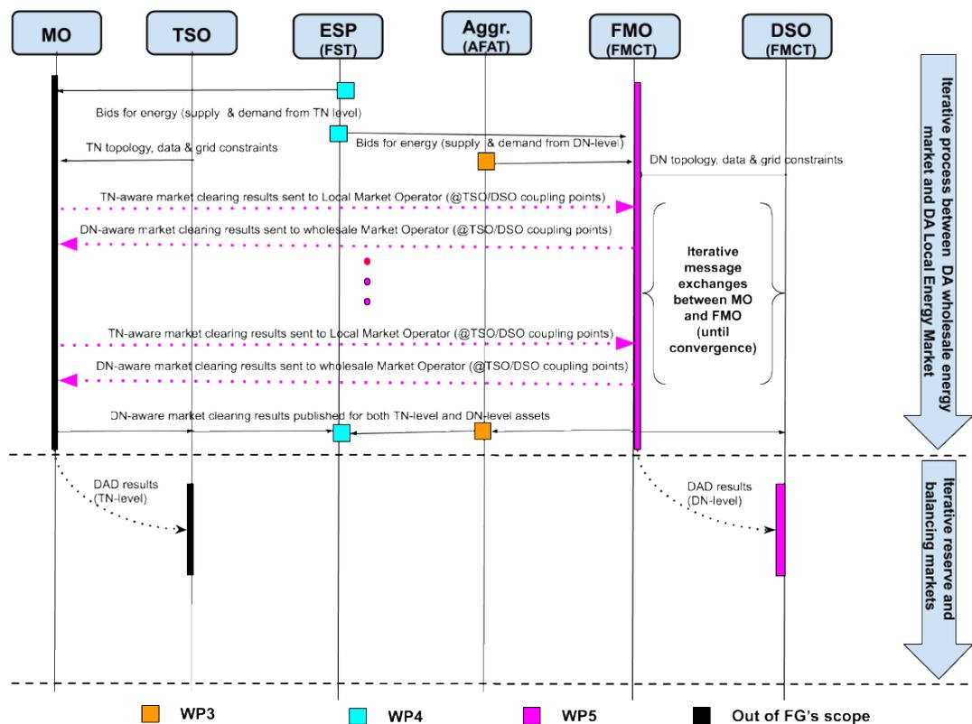
**Figure 11: Interactive DLEM (iterative message exchanges between MO and FMO until convergence)**
