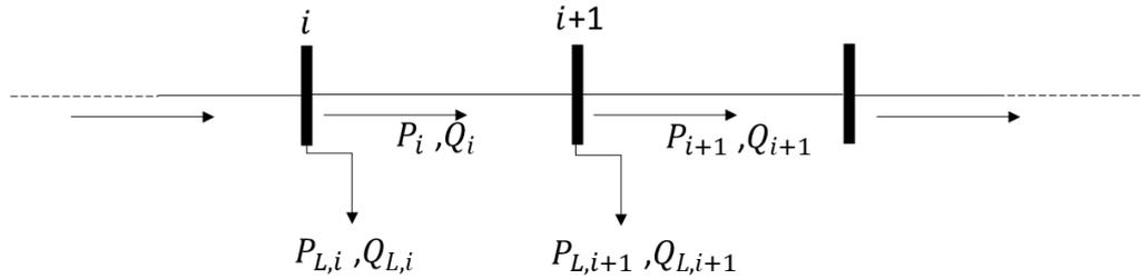
Figure 7: One line diagram of a radial network
